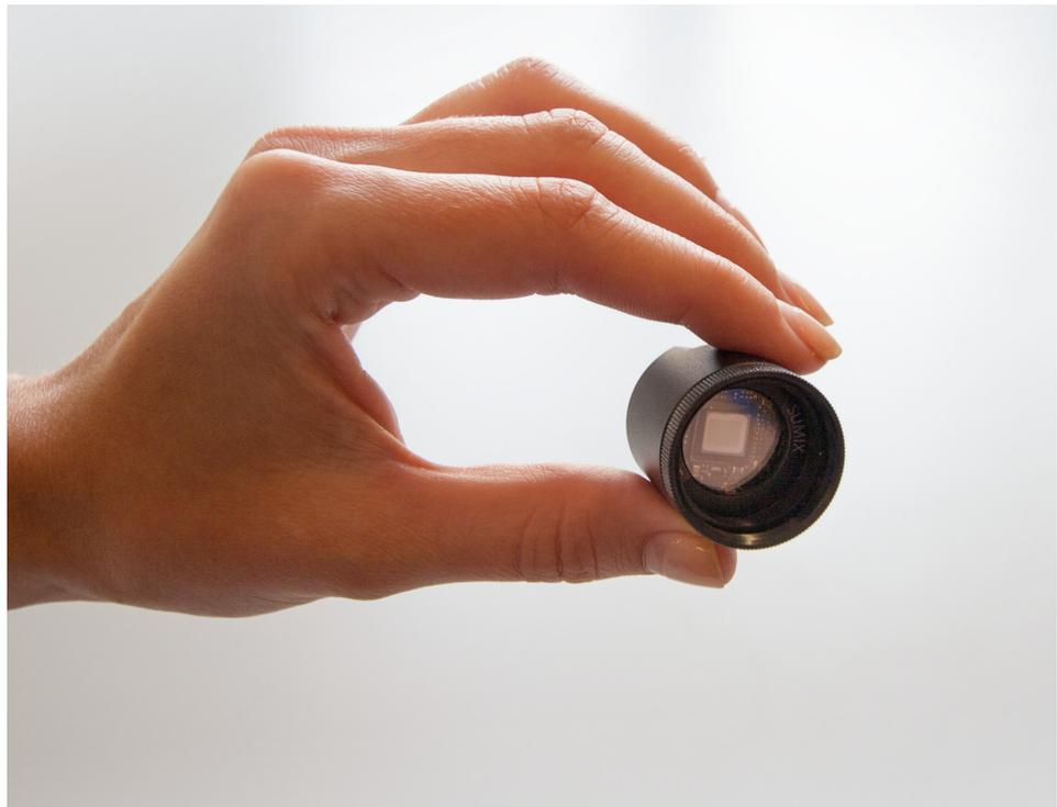
Note: It is recommended to screw in (as well as screwing out) the C-mount adapter, lens, or the Camera's cover when the Camera is facing down or when the Camera is in horizontal position – to prevent the sensor contamination.
