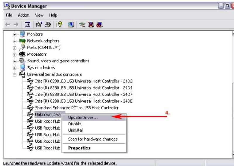
**Figure 2-17** Device Manager: Updating the SMX-M8x camera driver
