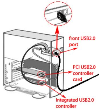
As shown on the picture above, the front USB2.0 port is connected to the USB Host Controller by long cables inside computer, meanwhile back USB2.0 port is connected directly to its controller at the back panel of computer.
