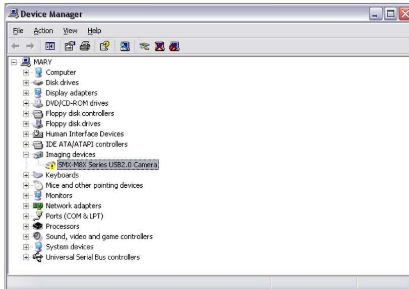
**Figure 2-15** Device Manager: the SMX-M8x camera with Warning status
