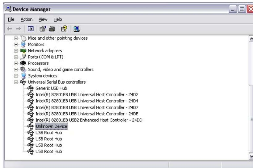
**Figure 2-16** Device Manager: the SMX-M8x camera is detected as Unknown device
